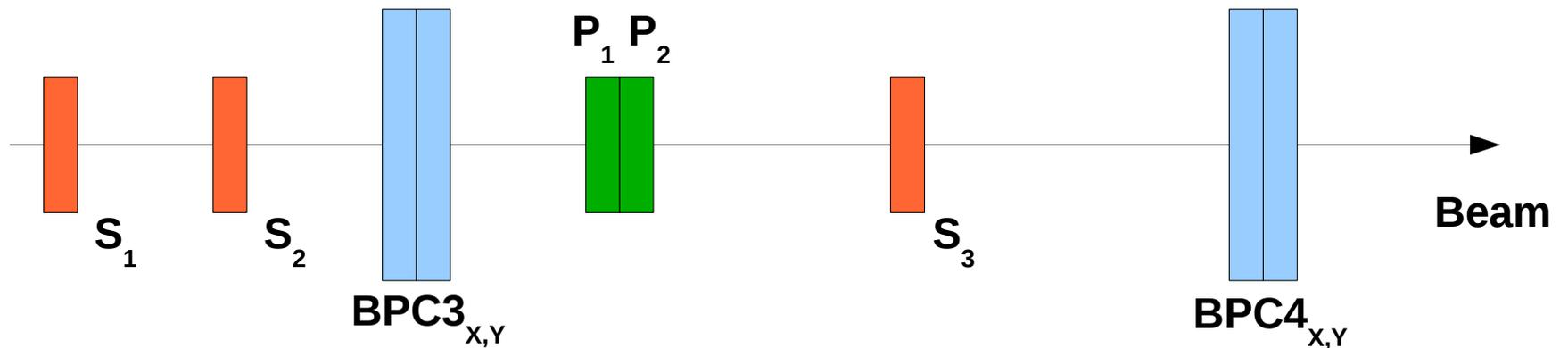
Prototype was placed between two doublets of proportional chambers (BPC). So it's possible to reconstruct trajectory of passing particle
