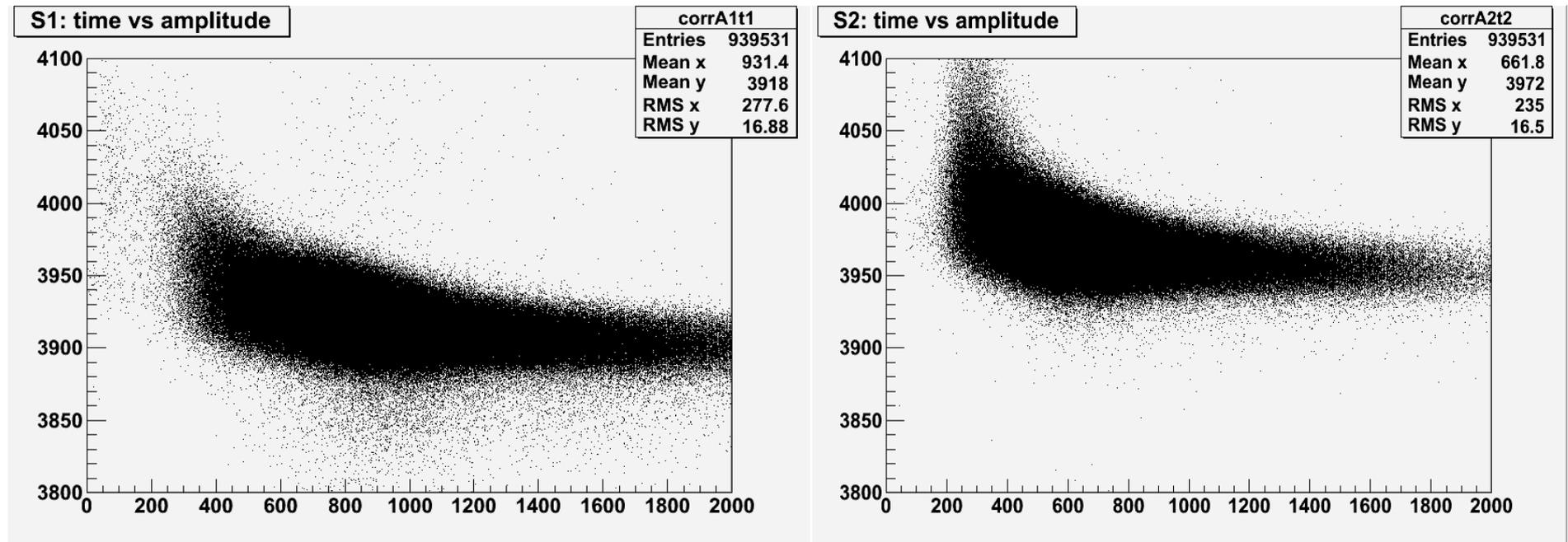
Fixed threshold discriminator introduce dependency on amplitude which worsens time resolution. So it should be taken into account.
