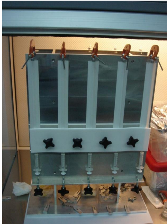
Figure 129 The fiber-bar gluing tool in action. Its back side is identical to the one shown. Glue is injected from bottom using syringe
