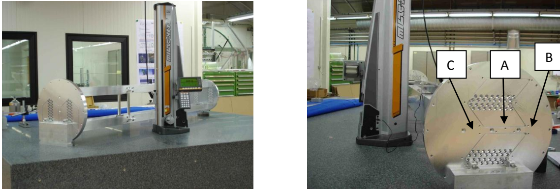
Figure 193. View of the prototype structure (left) and the measurement of the frame on the granite table.
