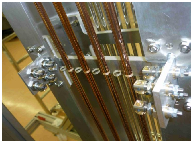
Figure 194. A view of four inserted straws supported by a spacer.
