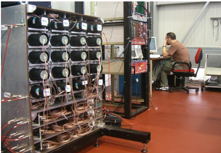
Figure 9 The Lead Glass Test Station is arranged in 4 columns of 5 blocks each. The top and bottom blocks of each column are fixed and used as a trigger for cosmic rays. The remaining 12 blocks are the detectors being tested.
