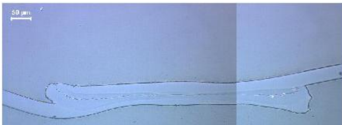
Figure 164. Cross section of a welded seam where the two sides of the strips are fused.
