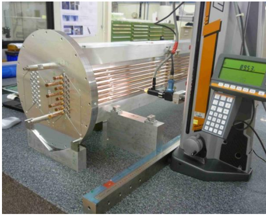
Figure 197. Measurement set up (left) and the distance between neighboring straws (right). The straws are kept at 2 bar absolute pressure 32 .
