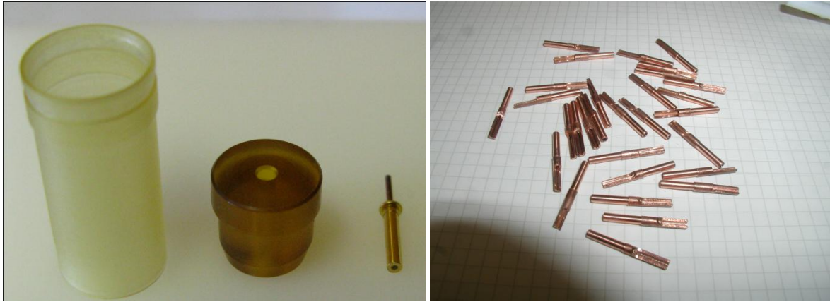
Figure 179. Details of the straw end-pieces are shown. The socket is glued between the straw and the structure (left). The connection plug pushes the petals of the web to the straw wall. The crimp-tubes connect the wire to the Kapton ® layer of the web circuit by crimping (left picture) or by soldering (right picture).
