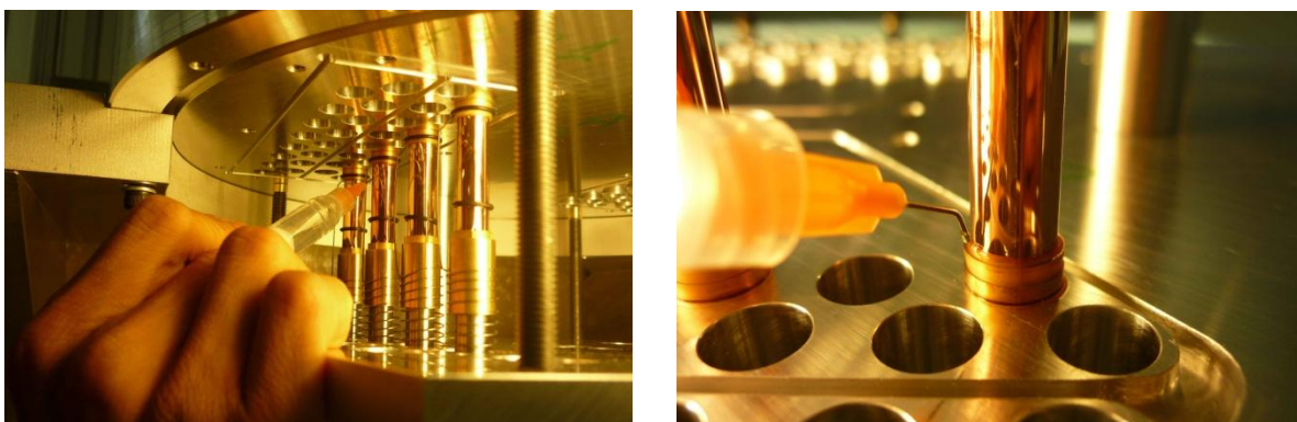
Figure 196. Bottom side gluing (left) and the gluing of the tope side (right).
