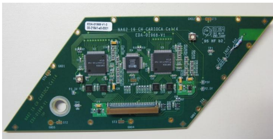
Figure 181. Front-End board (cover) with the two CARIOCA chips (front side). The cover is mounted on partition serves as a leak-tight roof for the gas manifold and feed through for gas, high-voltage and signal connections to the straws (back side).
