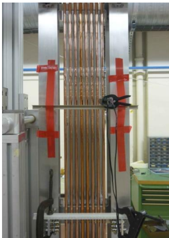
Figure 198. Set up in vertical position for straw tension measurements (left) and the measured tension (right).
