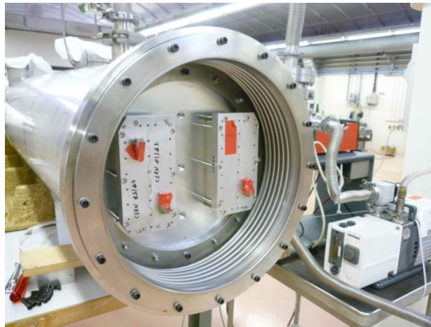
Figure 204. View of the far end with the metallic bellows for the vacuum and leak test. The two gas cells (without electronics) are visible in the center.
