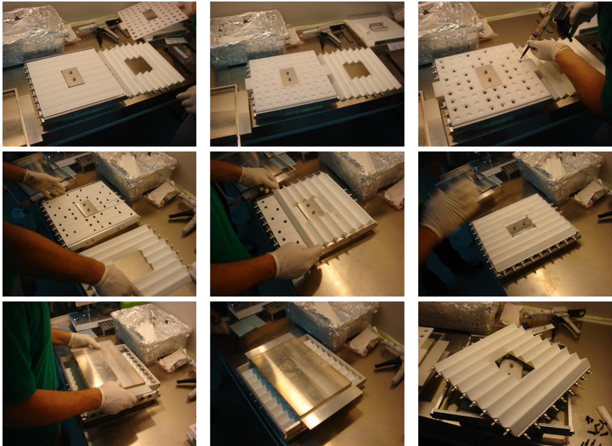
Figure 133 Assembling "First step": a) A half-layers is arranged on the jig, b) Teflon mask is aligned, c) Glue spots are applied, d) Mask is removed, e) f) Bars of the other half-layer are placed, g) h) second jig is applied on top to align last placed half-layer and to redistribute pressure, i) Half-module as appear the day after gluing
