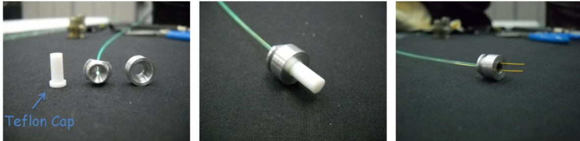
Figure 127 a) Connector in its parts b) Assembled connector c) Connector with SiPM
