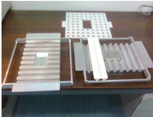
Figure 132 Jig used to align bars during gluing, on top Teflon mask to distribute glue spot
